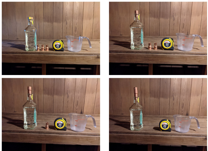
FIG. 3. Experimental materials and the Helmholtz resonator shown with (top-left) no extension, (top-right) one extension, (bottom-left) two extensions, (bottom-right) three extensions. The volume of the resonator was adjusted by filling the bottle with water to desired levels.
